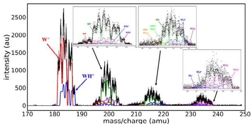
**Fig. 1.** Mass spectra of magnetron discharge with W target, generated in Ar/H<sub>2</sub> in presence of N<sub>2</sub> or O<sub>2</sub> impurities, recorded in the mass region 170 – 250 amu: black points and lines - experimental data, colored lines – fitting results
