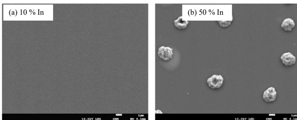
**Fig. 1** SEM images of (a) 10 at% In thin film with smooth, featureless surface and a (b) 50 at% In sample with imposed In-rich particle-like features onto a smooth background film.
