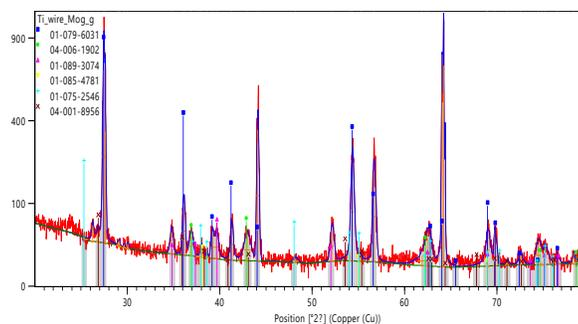
**Fig.2** XRD analysis of the titanium oxide thick titanium oxide layer from surface of the titanium wire: 01-079-6031-TiO<sub>2</sub>, 04-006-1902, 01-089-3074, 01-075-2546-TiO, 01-085-4781- Ti.
