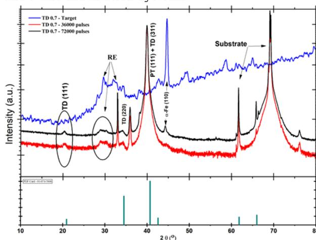
**Fig. 1** XRD patterns of TD 0.7 films deposited at 36000 and 72000 pulses.
