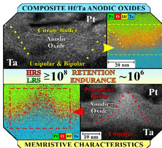
Fig. 1 Anodic memristor grown on Hf/Ta wedge library showing intrinsic nanostructuring of the mixed oxide.
