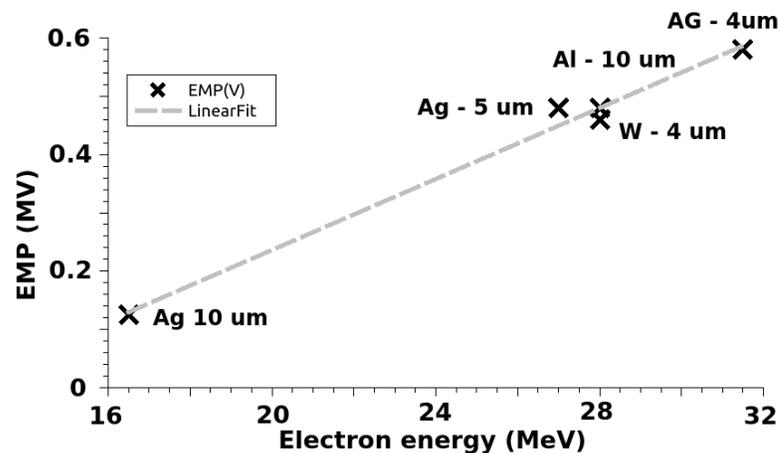
Fig. 1 Experimental correlation between (recorded) electron maximal energy and EMP (mediated) low frequencies amplitude .
