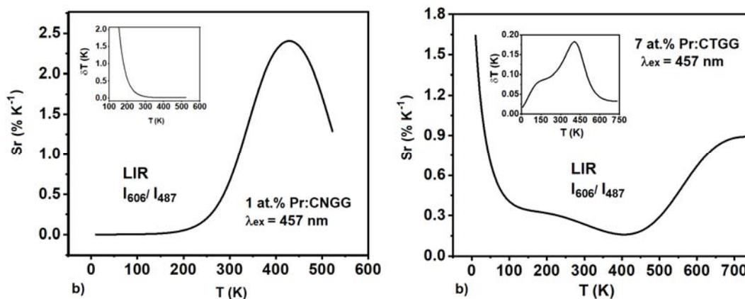
**Fig. 1** Relative thermal sensitivity curve  $S_r$  (b) as a function of temperature for 1at% Pr:CNGG (a) and 7 at% Pr:CTGG (b) phosphors.
