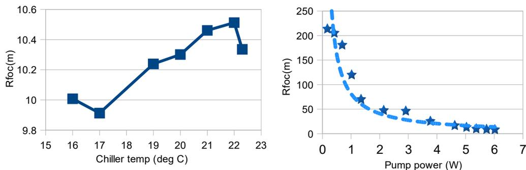
**Fig. 1.** Measured wavefront radius of curvature variation with circulating water temperature for the pump power of 5 W (Left) and wavefront radius of curvature variation with the pump power at circulating water temperature of 20 degree (Right).
