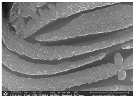
**Fig. 1** SEM image of the titanium wire irradiated with microwaves.
