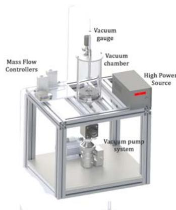
Fig. 1 Schematic representation of the plasma treatment setup
