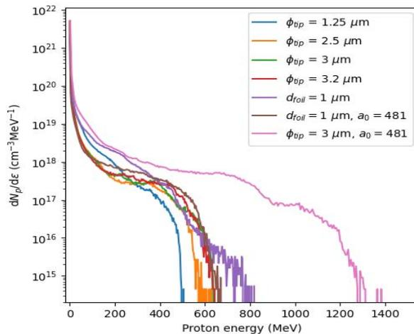
**Fig 1.** Proton energy spectrum for micro-cones with different tip diameters, the foil with the thickness of 1  $\mu\text{m}$  for  $a_0 = 215$  (everywhere where  $a_0$  is not specified in the legend) and  $a_0 = 481$  at the simulation time of 100 fs.
