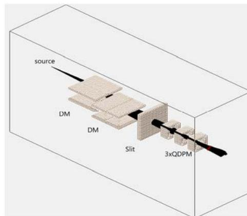
**Fig. 1** Setup overview of the proton beam steering system employing 2 dipole magnets (DP), a slit and 3 quadrupole magnets (QDPM).
