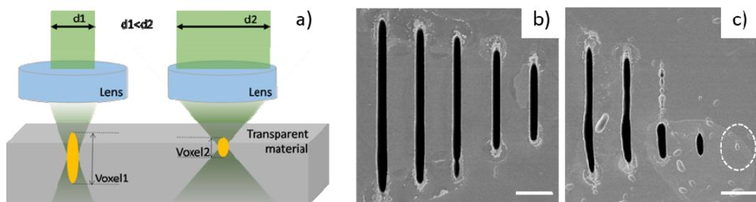
Fig.1. Voxel size variation in relation with laser beam diameter. a) Sketch of the voxel size in transparent materials; Embedded channels fabricated in Foturan glass by varying the picosecond laser beam diameter before the lens b) 3,5 mm ( $d_1$ ) and c) 11 mm ( $d_2$ ). The laser power was varied from 600 mW to 200 mW with 100 mW step in both configurations. The white dash circle from c) indicate the under-modification energy threshold. The scale bar is 100  $\mu\text{m}$ .
