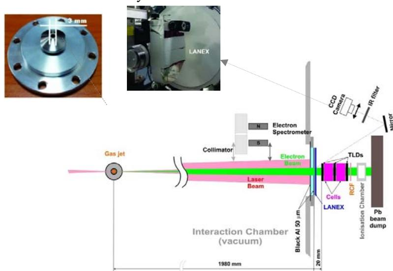
**Fig. 1** Schematic diagram of the laser-gas target experimental setup for the generation of accelerated electron beams and the irradiation of cell co-cultures *in vitro* [1].
