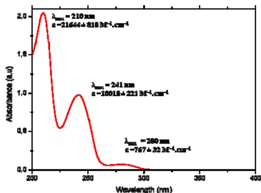
Fig. 1: Absorption spectrum of chlortoluron at  $98.7 \mu\text{mol.L}^{-1}$  (before plasma treatment)
