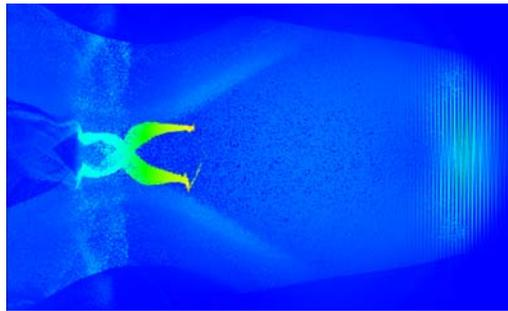
**Fig. 1** The bubble obtained for a plasma density  $2e^{18}(1+0.5 \cdot \sin(2\pi x/x_0)) \text{ cm}^{-3}$  after 900fs and with  $x_0=100 \mu\text{m}$ , shows a strong injection of electrons which perform high amplitude betatron oscillations.
