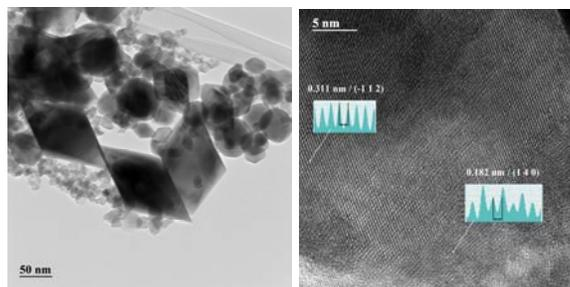
**Fig. 1.** TEM image of the deposited WO<sub>3</sub> nanoparticles.
