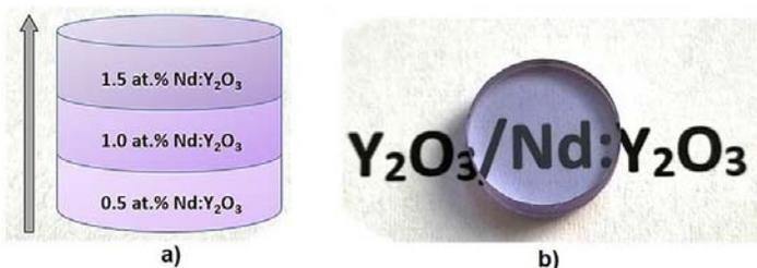
**Fig. 1** a) Schematic of a Nd:Y<sub>2</sub>O<sub>3</sub> ceramics with graded doping profile (the sample has three layers with increased Nd concentration). b) Image of 0.5-at.% Nd:Y<sub>2</sub>O<sub>3</sub>/1.0-at.% Nd:Y<sub>2</sub>O<sub>3</sub>/1.5-at.% Nd:Y<sub>2</sub>O<sub>3</sub> ceramic sample (thickness of 3 mm) obtained in our laboratory.
