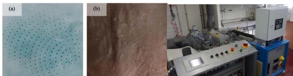
**Fig. 1** (a) BNC with a porous pattern; (b) BNC functionalized with lignin; (c) Semi-industrial atmospheric DBD plasma prototype.
