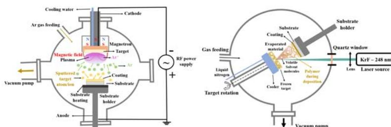
Fig. 1 Schematic representation of RF-MS (a) and MAPLE (b) experimental setup [2]
