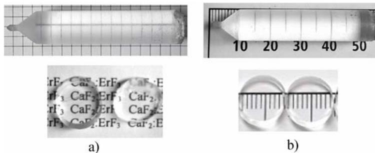
Fig. 1. Erbium doped  $\text{CaF}_2$  (a) and  $\text{BaF}_2$  single crystals (b).
