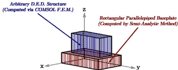
Fig. 1 Distribution of domains between the analytical solution and F.E.M. numerical solution.
