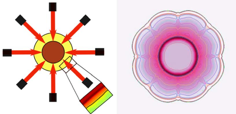
**Fig. 1** Scheme of a typical target for a direct laser-driven inertial fusion with nuclear combustion core and metallic shell. Inset presents electron density distribution on the surface of metallic shell generated upon the laser influence. Black line corresponds to margin of critical density region (Left). Preplasma temperature and density distribution in the irradiated target (right).
