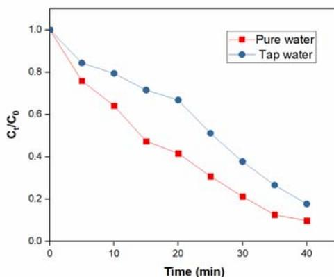
**Fig. 1** Degradation of CBZ in pure and Tap water: Needle to liquid surface distance 3.5 mm, HV = 10 kV, Frequency = 500 Hz, [CBZ]<sub>0</sub> = 25 mg.L<sup>-1</sup>
