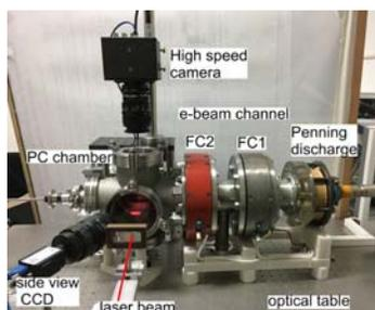
**Fig. 1** The laboratory platform for studying rotational dust flows in a PC irradiated by a  $\approx 10$  keV
