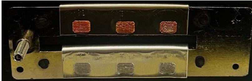
**Fig. 1** Example of laser welding application using different materials and thickness.
