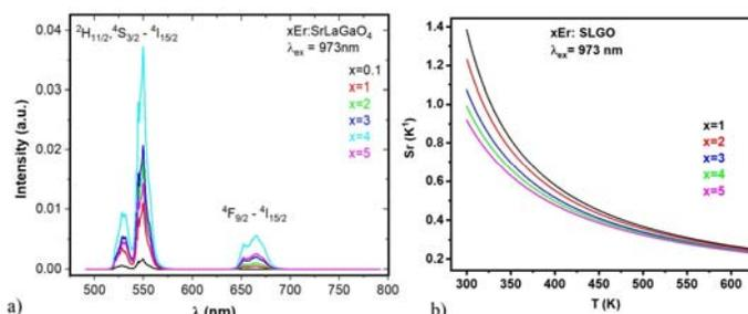
Fig. 1. Up-conversion luminescence of xEr: SrLaGaO<sub>4</sub> samples in the green and red domains under 973 nm excitation (a) calculated plots of Sr values function of temperature (b).
