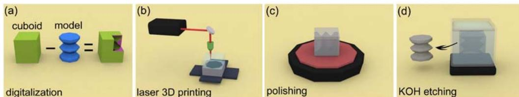
**Fig. 1** The ultrafast laser 3D printing process in glass.
