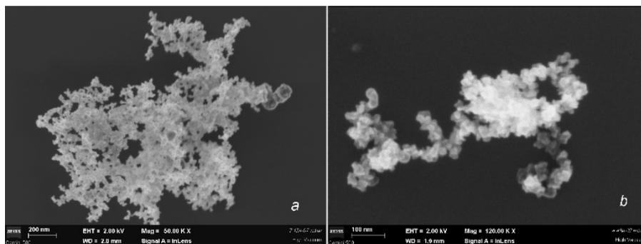
Fig. 1 (a) Boron nanoparticles obtained in MSGA adding small amounts of O<sub>2</sub> to Ar (a) and Kr (b).
