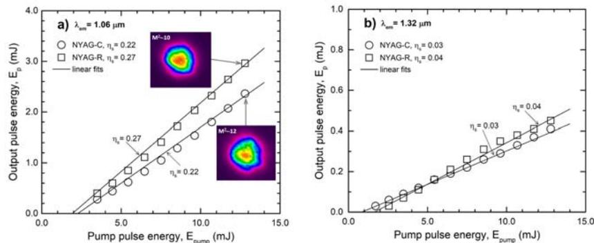
**Fig. 1.** a) The laser pulse energy,  $E_p$  at  $1.06 \mu\text{m}$  vs. pump pulse energy,  $E_{\text{pump}}$ ; OCM with  $T=0.05$ ;  $\lambda_{\text{em}}$ : wavelength of emission. The laser beam distributions are shown at the maximum  $E_p$ . b) The laser pulse energy,  $E_p$  at  $1.32 \mu\text{m}$  versus  $E_{\text{pump}}$ ; OCM with  $T=0.03$ .
