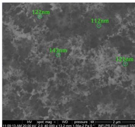
**Fig. 2** The SEM image of ZnO nanoparticles
