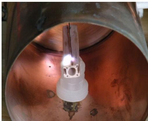
**Fig. 1** The image of plasma generated during interaction between microwaves and Zn wire
