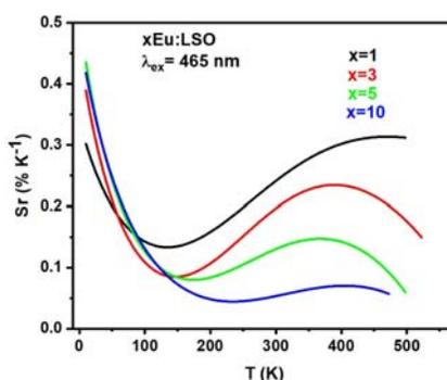
Fig. 1. The calculated curves of relative sensitivity Sr of  $\text{Eu}^{3+}$  in  $x\text{Eu}$ : SLO ceramic phosphors ( $x = 1, 3, 5$ , and 10).
