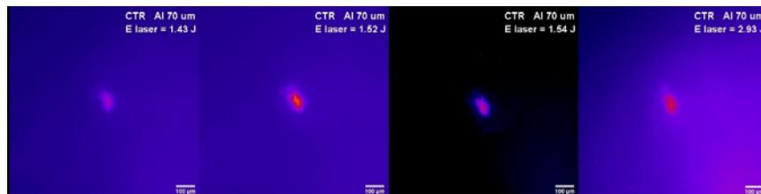
**Fig. 2.** CTR images recorded from Al foil at various laser energies
