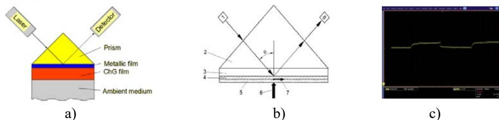
Fig.1. Characteristics of four layers SPR structure: **a)** SPR structure; **b)** 1- prism, 2 - immersion oil, 3 - glass slide, 4 - gold film 5 -  $\text{As}_2\text{S}_3$  amorphous film, 6 - irradiation beam; 7 - generated surface wave; **c)** experimentally measured changes of light reflectance due to film irradiation.
