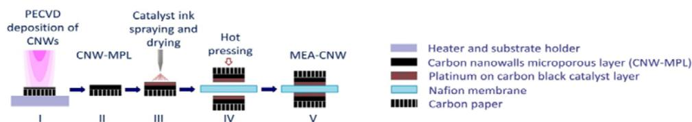
**Fig. 1.** Graphic illustration of the MEA fabrication: (I) N-doped CNW deposition on the carbon paper by PECVD techniques; (II) gas diffusion layer composed of CNW as MPL and carbon paper; (III) catalyst layer deposition by spraying the platinum ink on top of the MPL; (IV) hot pressing the two catalyst-loaded GDLs against Nafion- proton exchange membrane; (V) MEA\_CNW ready for tests.
