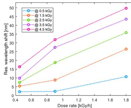
**Fig. 1** Dose-rate dependency of resonance wavelengths variations of an LPG exposed to a Co-60 gamma source
