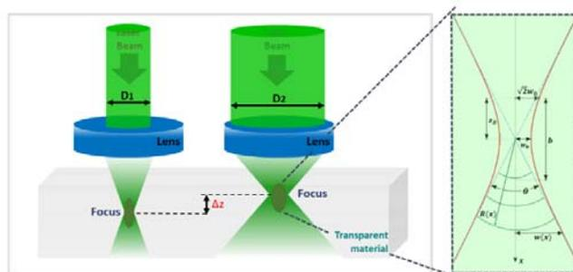
**Fig. 1.** Conceptual representation of the laser beam focalization in Foturan glass, showing the focal distance change ( $\Delta z$ ) induced by the expanded diameter of collimated laser beam to provide the Rayleigh range  $z_R$  and the confocal parameter  $b$  ( $R(x)$  - radius of the curvature of the wavefront,  $w(x)$  - the gaussian spot size,  $\theta$  - full divergence angle)
