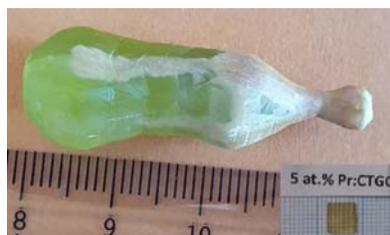
**Fig. 1.** As-grown Pr:CTGG single crystal. The inset shows a polished crystal sample cut from the grown crystal.
