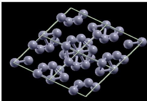
Fig. 1 The  $\alpha$ -boron crystalline structure studied using density functional theory.
