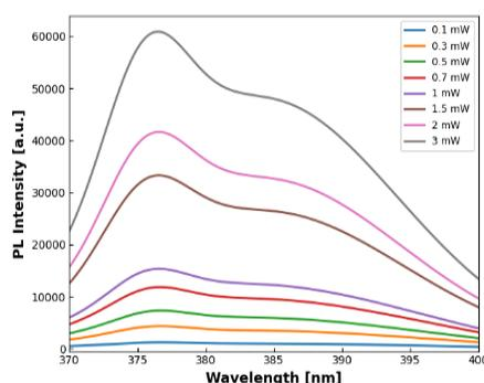
Fig. 1. Power dependent PL spectra of ZnO heterostructures at room temperature
