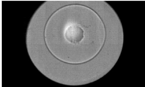
**Fig. 1** Blast wave formed due to laser-induced breakdown at  $E_{inc} = 100$  mJ and  $P_0 = 1000$  mbar in Compressed Air,  $\Delta t = 5.6805 \mu s$
