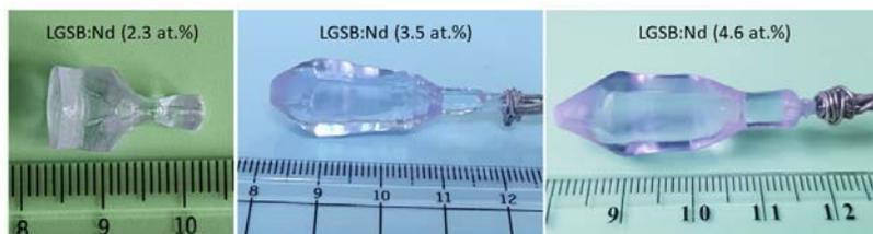
Fig. 1. Photos of Czochralski-grown Nd:LGSB-type crystals.
