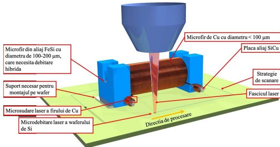
Fig. 1 Microcoil with Cu winding and FeSi core, mounted on Si support.
