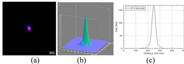
**Fig. 1.** Focal spot classically measured with the focus microscope (a) Image of the focal spot; (b) 3D spatial profile of the focal spot; (c) 2D profiles of the focus on two orthogonal directions
