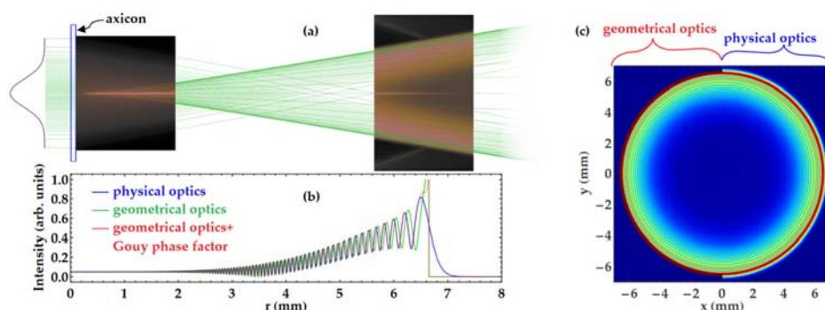
**Fig. 1** (a) Propagation of the Gaussian beam ( $w_0 = 2.5$  mm) longitudinal view. (b) Radial intensity profile of the beam at 500 mm from the axicon that was computed using physical optics (blue), geometric optics (green), and geometrical optics considering the additional Gouy phase along the ray. (c) Transverse profile of the beam at 500 mm from the axicon both physical optics (right) and geometrical optics (left).
