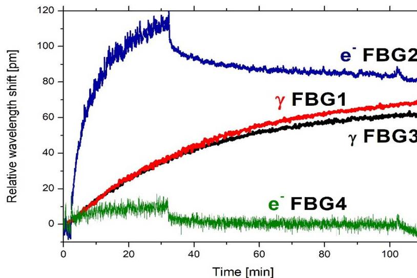
**Fig. 1** The relative wavelength shift of four FBG sensors for two different types of radiation.
