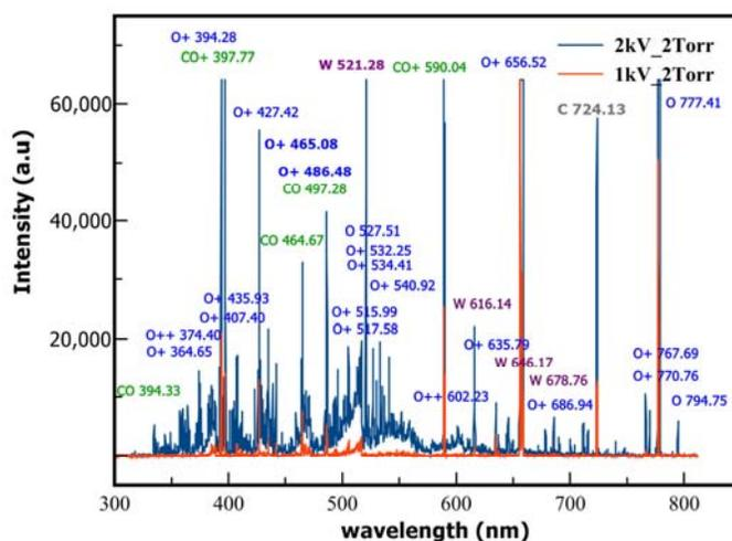
Fig. 1. Full emission spectra captured for two discharge voltages, 1 kV (in red) and 2 kV (in blue), at a CO<sub>2</sub> pressure of 2 Torr [1].
