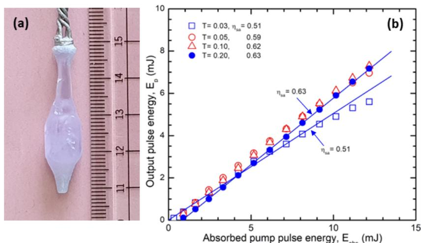
Fig. 1 Photo of the as-grown Nd:LYSB crystal (a) and quasi-CW laser emission performances at  $1.06 \mu\text{m}$  of the Nd:LYSB crystal (b).
