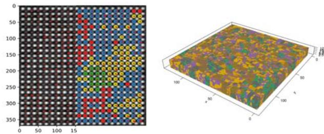
**Fig. 1.** STEM atomic displacements and K-means predicted domains (left), Phase Field simulations of ferroelectric domains (right)
