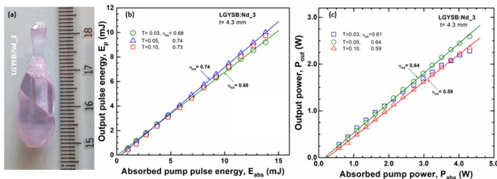
**Fig. 1** As-grown LGYSB:Nd<sub>3</sub> crystal (a), laser pulse energy,  $E_p$  versus absorbed energy of the pump pulse,  $E_{\text{abs}}$  and (c) output power,  $P_{\text{out}}$  versus absorbed pump power,  $P_{\text{abs}}$  for LGYSB:Nd<sub>3</sub> crystal. The near-field distribution of the laser beam is shown in the figure inset, at the highest output level.
