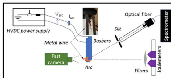
Fig. 1 Experimental set up (top view)
