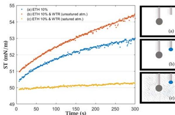
**Fig. 1** Surface tension behaviour of a 10 % ethanol drop ( $V=12 \mu\text{l}$ ) (a) without presence of other drop, (b) in the proximity of a water drop in unsaturated atmosphere, (c) saturated atmosphere.
