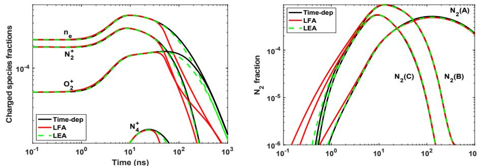
**Fig. 1.** Time-evolution of representative charged (left) and neutral (right) species for a nanosecond discharge in air at  $p=10$  Torr: (—) exact MC solution; (—) local field approximation; (---) local energy approximation
