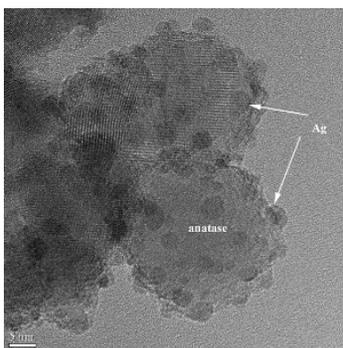
Fig. 1 HRTEM image for the TiO<sub>2</sub> based sample loaded with Ag
