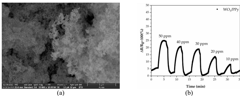
**Fig. 1** (a) SEM image of PPy/WO<sub>3</sub> structure (b) Time dependent response obtained at 22±1°C of a sensor with WO<sub>3</sub>/PPy active layer.
