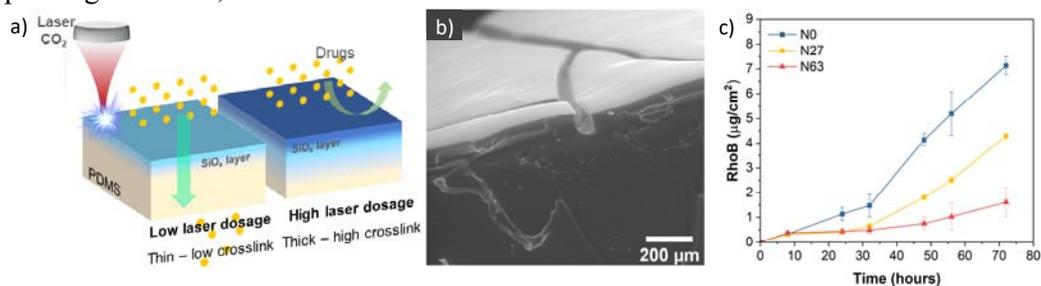
**Fig. 1** a) Schematic representation of diffusion barrier layer, b) SEM image of the barrier layer interface on sample N45
