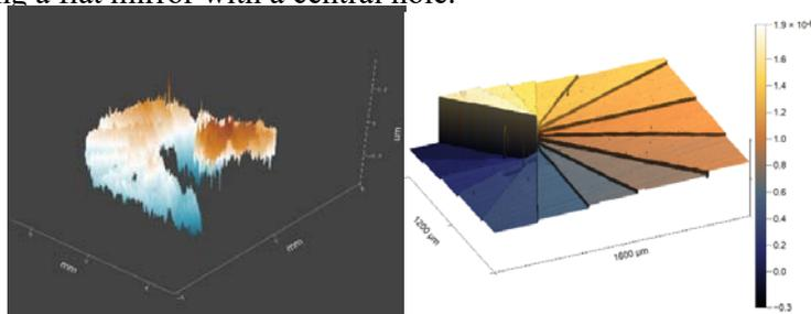
**Fig. 1** (Left) Measured 3D full-aperture (80.64 mm x 108.96 mm) helical wavefront produced by a 6'' spiral phase plate with topological order  $l=1$ ) with a high resolution wavefront sensor, and (Right) real-time profilometer measurement of a  $10 \text{ mm}^2 \times 10 \text{ mm}^2$  optical profile image after data post-processing.
