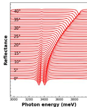
**Fig. 1.** Angle resolved reflectance from a typical microcavity in strong coupling regime.
