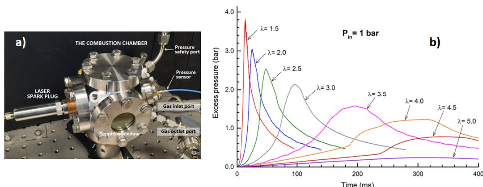
**Fig. 1 a)** The constant-volume combustion chamber and a single-beam laser spark plug.
