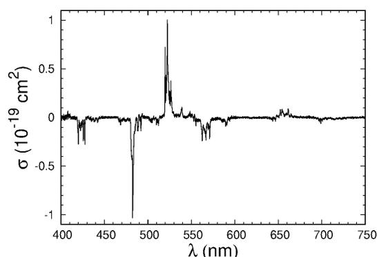
Fig. 1 ESA spectrum of Er:Y<sub>2</sub>O<sub>3</sub>, calibrated in cross-section units. Up: lines corresponding to ground-state absorption; down: lines corresponding to ESA.
