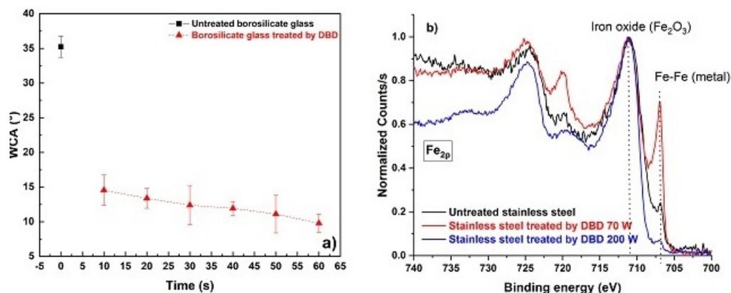
**Fig. 1.** a. variations of water contact angle (WCA) with respect to the DBD plasma treatment time of glass, b. XPS analysis of stainless steel treated by DBD plasma treatment at different powers.
