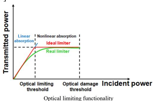
For the ideal OL the transmitted power/intensity has a linear increase for incident power/intensity up to the OL threshold, remaining constant after this. For a real OL, the transmitted power/intensity depends nonlinearly on the incident one, being described by a saturation curve.
