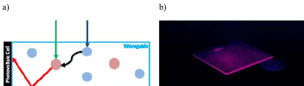
Fig. 1 (a) Edge-on schematics explaining the basic principle of a luminescent solar concentrator. (b) Image of the optimised device excited with ultraviolet radiation.
