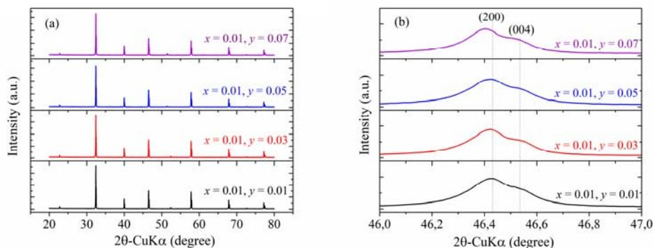
**Fig. 1** X-ray diffraction spectra for  $\text{Sr}_{1-3(x+y)2}\text{Er}_x\text{Yb}_y\text{TiO}_3$  powders calcined at 1000 °C, 2h in air: XRD patterns (a) and detail (b) for  $x = 0.01$ ,  $y = 0.01$ -0.07.
