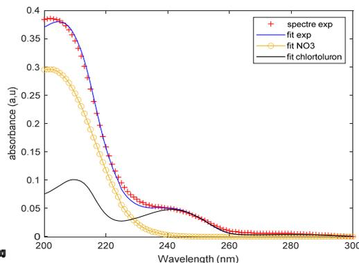
Fig. 2: Comparison of experimental spectra, global fit, nitrate ion fit and chlortoluron fit for chlortoluron solution treated by plasma jet ( $t= 20 \text{ min}$ ,  $V=50 \text{ mL}$  and  $[\text{chlortoluron}]= 98.7 \mu\text{mol.L}^{-1}$ )
