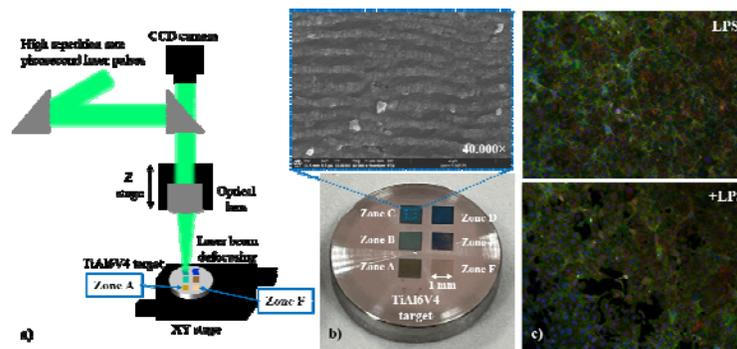
**Fig. 1** (a) Setup for laser-texturing. (b) Image of TiAl6V4 irradiated with different laser doses and SEM image of the Zone C (used for cell cultures). (c) Immunofluorescence images of hGEPiCs in contact with laser processed TiAl6V4, in the presence (+LPS) or absence (-LPS) of an inflammatory process. Proteins visualization: actin (green), vinculin (red), nucleus (Hoechst-blue).
