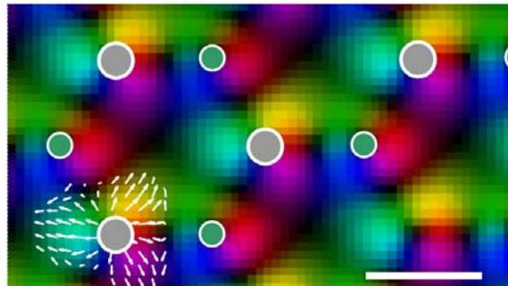
**Fig. 1** DPC-STEM image of the interatomic electric field distribution in a pristine WSe<sub>2</sub> monolayer with central W and Se atomic positions marked in grey and in green, respectively. Colours represent the direction and strength of electric fields, partially also indicated by vectors. The scale bar is 2 Å.
